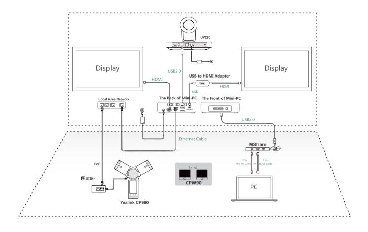
For convenience, we recommend that you connect a wireless USB dongle to the back of the Mini-PC to use mouse and keyboard to manage devices.
