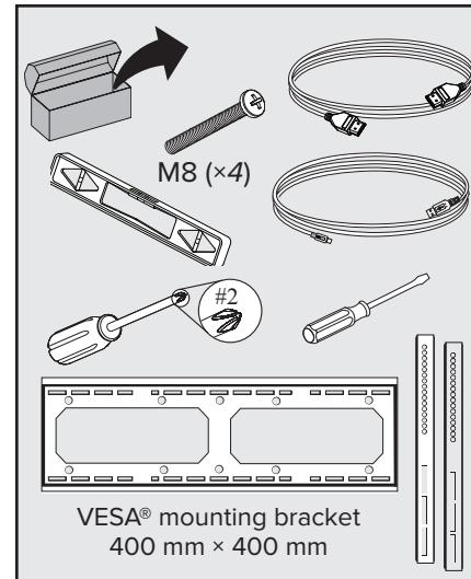
**!** Do not move or mount the interactive flat panel by connecting rope or wire to its handles. Because the interactive flat panel is heavy, rope, wire or handle failure could lead to personal injury. Use only VESA®-approved mounting hardware.
