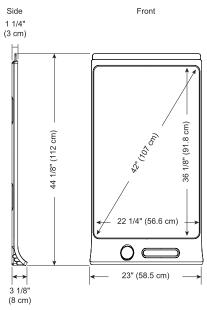
Weight 35 lb. (16 kg) Shipping dimensions One unit on a pallet 47 1/4" × 25" × 5 3/8" (119.9 cm × 63.5 cm × 13.6 cm) Shipping weight One unit on a pallet 47 lb. (21.3 kg) Seven units on a pallet 270 lb. (122.5 kg)
