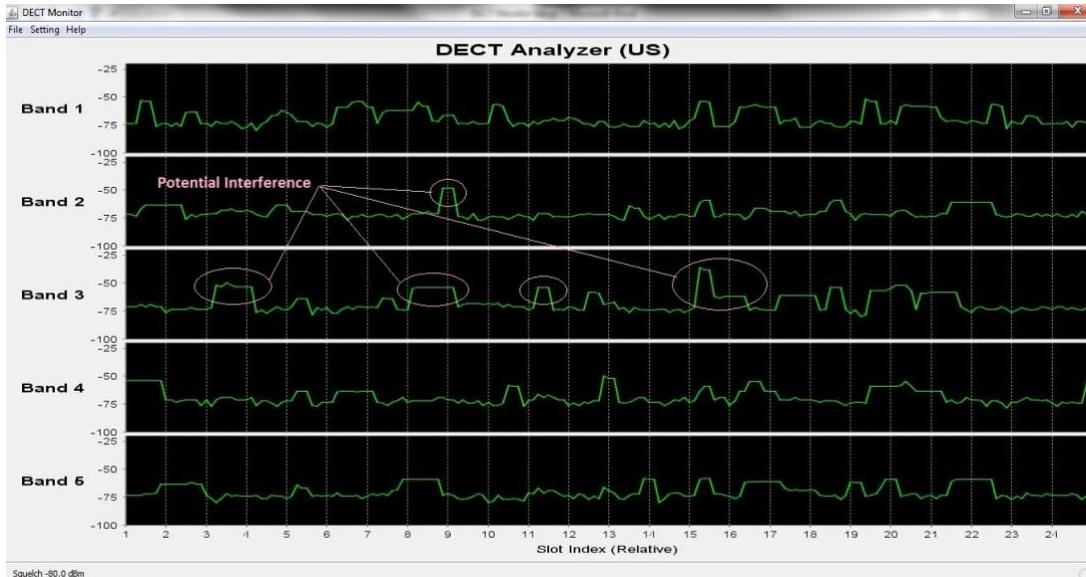
Below is a scan taken with less than (5) five interfering devices, which would be conducive to normal operation of HD products.
