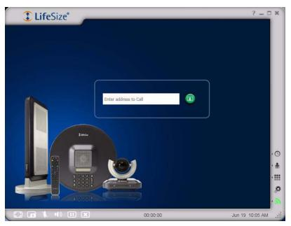
LifeSize Desktop runs on a Windows XP or Vista personal computer with a USB headset or other speaker and microphone, and a USB webcam. Desktop users outside the enterprise network firewall can call users inside the firewall. Refer to "Enabling Firewall Traversal" on page 15.
