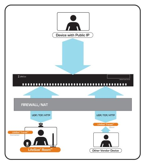
The default configuration of LifeSize Transit Server includes a Media Server and a Signalling Server (Proxy Server) enabled within the same 1U device. Optionally, you can decouple the Signalling Server from the Media Server enabling multiple Media Servers to work directly with a single Signalling Server.
