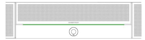
• Muting the microphone and speaker turns the two outer segments of the status bar red.
