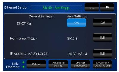
The "Ethernet Setup" menu displays current settings, such as whether DHCP is on or off, the touch screen's *Hostname* and its *IP Address*. There are controls for turning *DHCP* **On** or **Off** as well as controls which allow editing of the *Hostname* and *IP Address*. This menu also contains *Link* and *Ethernet* indicators to show the status and activity of the Ethernet connection. Other controls on this menu are explained in paragraphs that follow.
