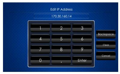
Use the keyboard to enter the new IP address. Touch **Clear** to clear any previous entry, **Backspace** to delete the last digit, **Enter** to save a new entry or **Cancel** to return to the previous screen.
