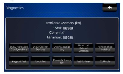
The "Diagnostics" menu displays the *Available Memory* and contains controls to **Show Hardware Configurations**, **Show Cresnet Devices**, **Show Message Log**, **Show Last Reboot Message** and **Performance Statistics**. In addition there are controls to open various test screens and to initiate touch screen calibration. These are explained in the paragraphs that follow.
