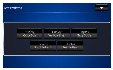
The "Test Patterns" menu contains buttons for selecting the different available test patterns: Display Color Bars, Display Vertical Lines, Display Gray Scale, Display Grid Pattern and Display Test Pattern.
