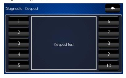
The "Diagnostics - Keypad" screen can be used to test the function of the hard key push buttons on either side of the screen. When a button is pressed, its corresponding indication on the screen lights.
