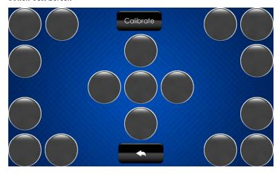
The touch test screen contains a **Calibrate** button to initiate touch screen calibration and a **Return** button to return to the "Diagnostics" menu.
