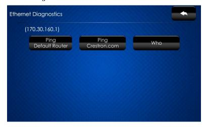
The "Ethernet Diagnostics" screen provides controls for verifying connections. Touch **Ping Default Router** to verify connection to the router. (The screen displays a "Passed" message to show successful connection.) Touch **Ping Crestron.com** to verify connection to an external DNS server.
