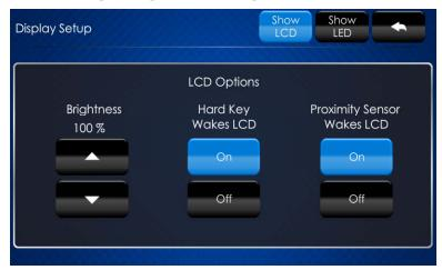
The LCD Options include controls to adjust screen Brightness along with **On** and **Off** controls for Hard Key Wakes LCD and Proximity Sensor Wakes LCD.
