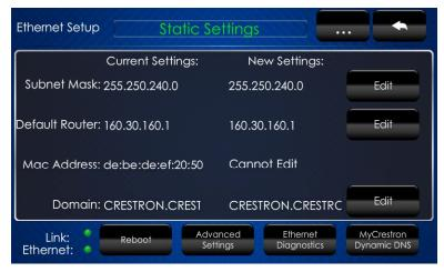
The additional parameters are *Subnet Mask*, *Default Router*, *Mac Address* and *Domain*. For *Subnet Mask*, *Default Router* or *Domain*, touch **Edit** on the right side of the menu to open on-screen keyboards like the ones described above.
