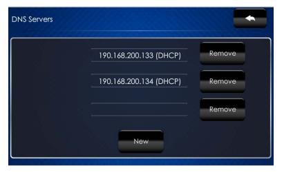
The "DNS Servers" screen provides controls for adding or deleting the IP addresses of DNS (Domain Name System) registered computers on the network. To add a server's IP address, touch **New** to open an on-screen keyboard.
