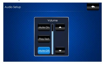
The "Audio Setup" screen provides controls for muting (or unmuting) the audio, adjusting *Volume* and playing a test .wav file.
