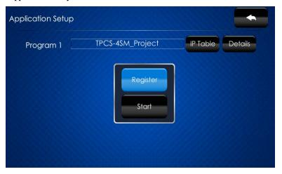
The "Application Setup" screen has controls to enable or disable the user program from running when the device boots and to restart the program.
