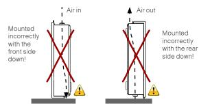
**NOTE:** Incorrect mounting as shown above will not allow for enough ventilation through the codec.
