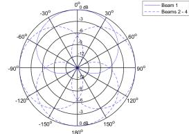
TTM-X Polar Responses at Center of Tracking Zones Patterns Shown at 2000Hz at an elevation of 30° from Table
