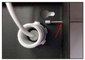
Figure 20 End-stop Installation
