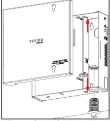
Figure 19 Seismic Cable Installation
