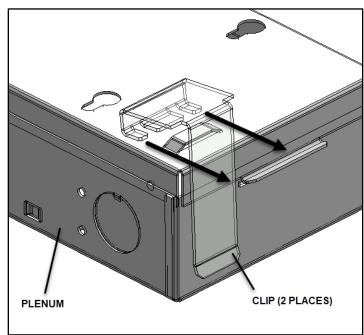
Figure 16 Clip Installation
