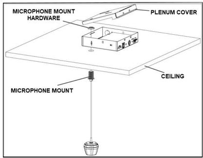
Figure 12 Above-Ceiling Tile Installation Option
