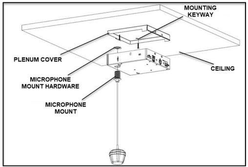
Figure 14 Ceiling Installation Option
