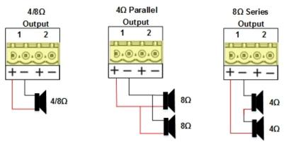
Figure 7 Amplifier speaker wiring (TCM-1A only)
