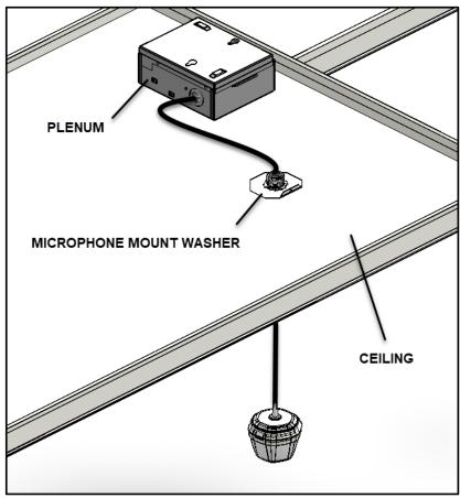
Figure 13 Alternate Above-Ceiling Tile Installation Option
