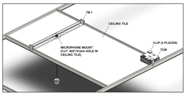
Figure 17 TB-1/TCM Corner Installation
