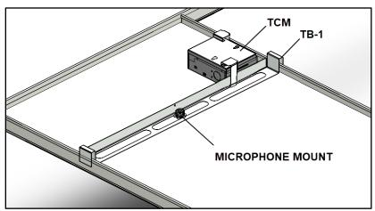
Figure 18 Alternative TB-1/TCM Installation
