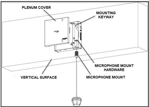
Figure 15 Vertical Surface Installation
