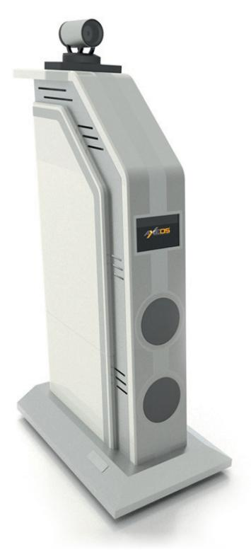
XELYS is a mobile videoconferencing solution. Its aim is to bring audio and videoconferencing technology into underequipped locations. When connected to a videoprojector, it offers a genuine and efficient videoconferencing solution.
