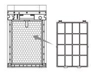
X The side with a handle should be placed outwards.
