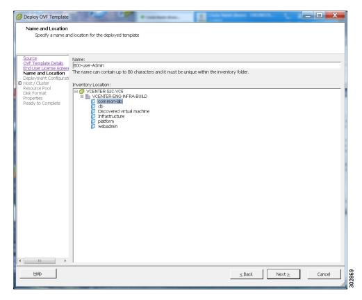
**Step 7** From the drop-down list, select the virtual machine for your system size then select **Next**. Be sure to deploy the Admin virtual machine before any other virtual machines in your system.
