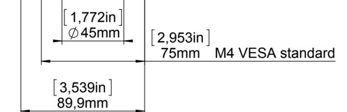
mounted on a ceiling mount complying with the VESA standard
