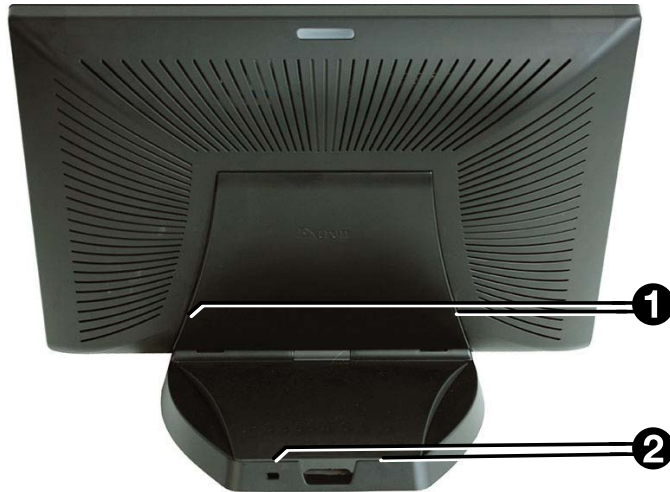
Figure 23. Remove the Back and Base Covers
