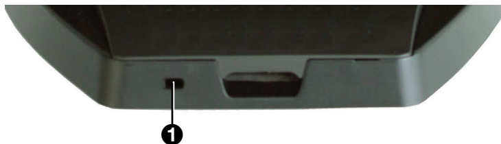
Figure 25. TLP Pro 1220TG Base, Showing Kensington Security Slot
