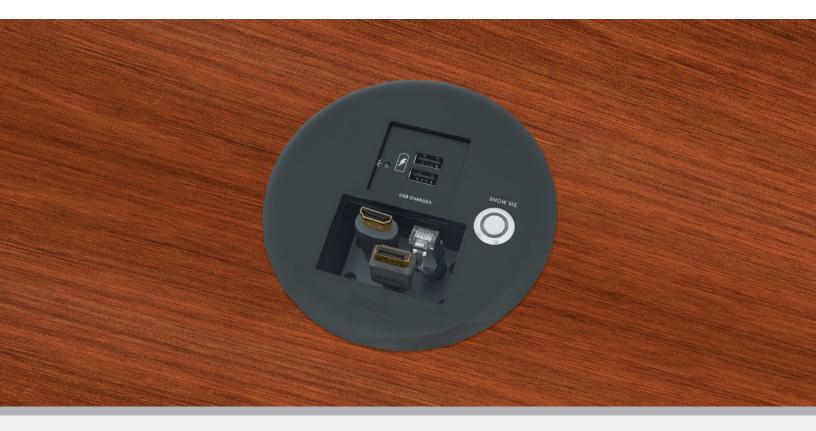
The Cable Cubby® 100 is a compact, furniture-mountable cable access enclosure for AV connectivity and AC or USB power. Its convenient round design eliminates the need to measure or use a routing template, making installation quick and easy using a standard four inch hole saw. The space-saving design is ideal for lecterns or any application where a single user access point is required.
