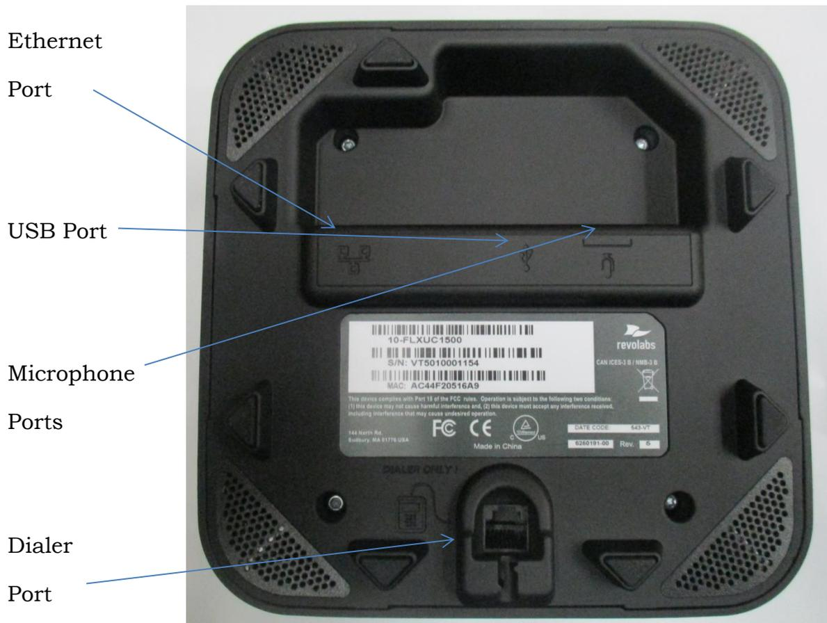
Figure 3: FLX UC 1000, Connector View
