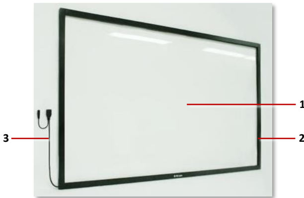
Example touch screen overlay: PQ Labs G4 Series Multi-touch screen. 1 Ultra-smooth toughened glass. 2 Infrared transmitters and receivers built into the surround frame. 3 USB cable.
