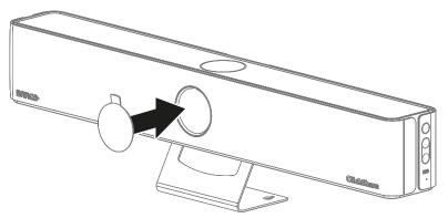
Image 4-3 Attach direction for the lens cover
