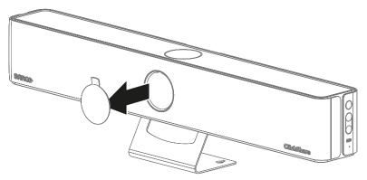
Image 2-2 Example of removal of the lens cap
