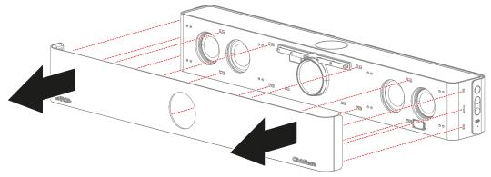
Image 5-4 Location of all fixations and direction to pull the front cover
