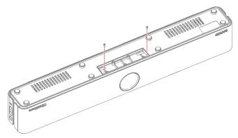
Image 5-2 Location of the two front cover screws to unscrew
