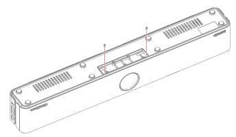
Image 5-9 Location of the two front cover screws to tighten
